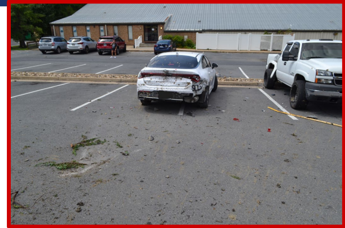
Flyrock damaged vehicles and pavement - August 2022
